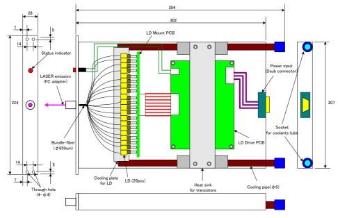
Dimensions are in millimeters.
